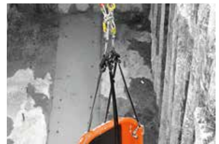
The self-redundant harness with adjustable patient safety allows for rescue with a vertically suspended stretcher.
